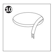
Caution: Careful attention should be made to cut within the hole diameter for the best fit Pull electrical wire through
