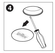
Remove cardboard cover. Use a small screwdriver to clean the inside lip of the trim collar of any excess drywall mud
