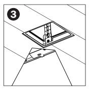
Install wood ceiling. Hole size **3-1/32" to 3-1/16"** Square. Can use adapter ring as template. **Do not use baseplate as hole template.**
