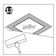
Apply thin coat of plaster mud onto trim collar and fibre mesh, using collar lip as the height guide. For best results feather mud 12" from edge of lip
