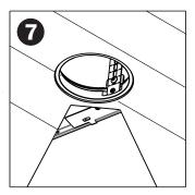
Install wood ceiling. Hole size 3-1/32" to 3-1/16" Diameter. Can use adapter ring as template. **Do not use baseplate as hole template.**
