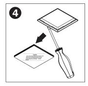
Remove cardboard cover. Use a small screwdriver to clean the inside lip of the trimless frame of any excess drywall mud
