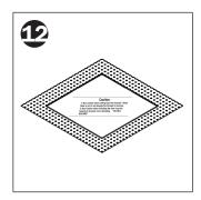
Apply factory supplied fibre mesh over trim collar edge. Insert cardboard cover into opening
