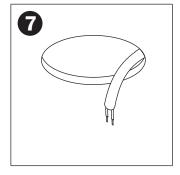
Caution: Careful attention should be made to cut within the hole diameter for the best fit Pull electrical wire through
