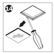
Remove cardboard cover. Use a small screwdriver to clean the inside lip of the trim collar of any excess drywall mud
