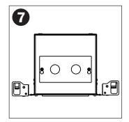
Remove the Knock outs and make appropriate electrical connections.
