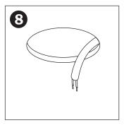
Caution: Careful attention should be made to cut within the hole diameter for the best fit Pull electrical wire through newly cutout hole
