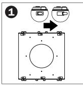
Slide and click tabs onto plate. Ensure mounting holes line up for step 2a.
