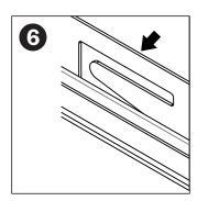
To lock baseplate in place, bend tab with pliers over hanging bar.
