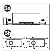
5a — Position trim hole to desired location by sliding housing
