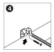
Line up bottom edge of hanging bars with bottom of wood joist and hammer in tabs. Nail or screw hanging bars into place
