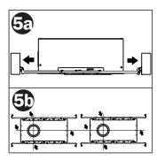
5a — Position trim hole to desired location by sliding housing
