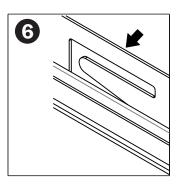
To lock baseplate in place, bend tab with pliers over hanging bar.
