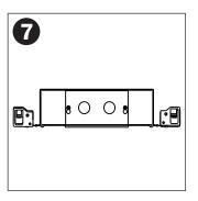
Remove the Knock outs and make appropriate electrical connections.
