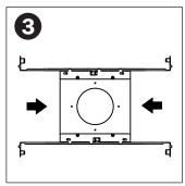
Slide hanging bars onto assembled base plate.
