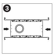
Slide hanging bars onto housing base plate
