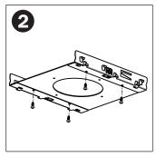
Align holes and screw brackets to base plate.
