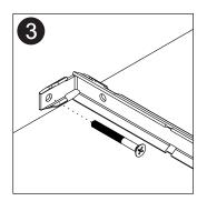
For added security install a nail or screw through the hole.
