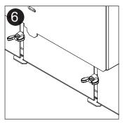
When fixtures is in its desired position, secure in place by tightening wing nuts.
