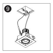
Clip safety hook onto latch on side of trim. Connect wire connector(s) from trim to housing.
