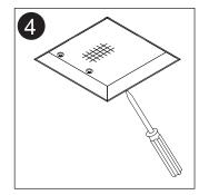
Use a small screwdriver or straightedge to clean the inside edge of the trimless frame of any excess drywall mud.
