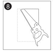
Mark approximate fixture location in ceiling. Cut open using hole as your guide.
