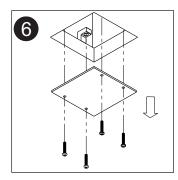
Remove protective cardboard cover. Screws not required further.
