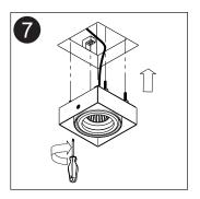
Insert trim assembly into place and secure with (4) captive screws.
