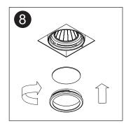
To Install an optional glass lens, twist counter-clockwise to release front ring, turn ring until tabs line up & ring drops out. Install glass lens into face ring. (Glass Lens ordered separately)
