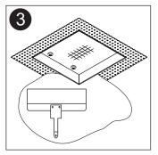
Apply thin coat of plaster mud onto trimless frame, using frame lip as the height guide. For best results feather mud 12" from hole edge.
