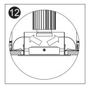
With trim pushed into ceiling, push the end of each clip outwards until they lock in place.
