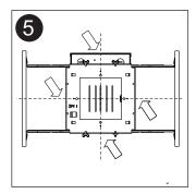
To line up a row of fixtures, use centering holes on either side of base plate.
