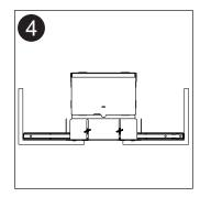
Position base plate to desired location by sliding left/right or up/down.
