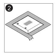
Apply fibre mesh tape (provided) over trimless frame edge. Remove excess tape.
