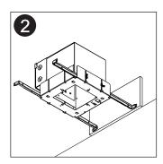
For wood joints bend end tabs 90 degrees.
