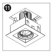
Compress trim clips flat to side of fixture, and then insert trim into ceiling cutout.
