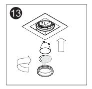
Remove protective film over adapter. Re-install reflector, adapter and face ring.
