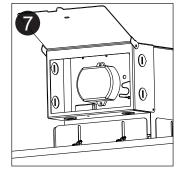
Unhinge lid of electrical box & connect input power to Primary of transformer.
