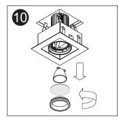
Before installing trim, remove face ring, adapter & reflector by turning all parts counterclockwise.
