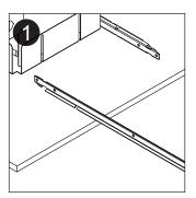
Slide hanger bars into base plate in the desired direction.
