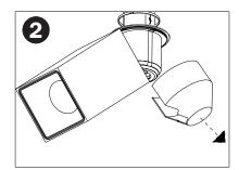
See C3SS-3C Junction box mounting (Step 1 & 2 ). Tilt cylinder to expose mounting/assembly cover.
