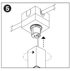
Ensure secondary leads are connected (+)(-) with lever locks. Twist cylinder clockwise to lock to the mounting assembly. If cylinder is not aligned with canopy, unlock from mounting assembly, rotate cylinder 120deg and lock again.
