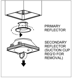
To service or change the reflector. Press suction cup onto glass and pull. Hold onto cylinder while pulling if possible. Contact factory for suction cup procurement. Rotate the primary reflector 45° counter clockwise to release.
