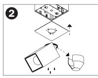
Place canopy lid inside of canopy. Align three larger size mounting holes with tapped holes on inside plate. Pull to remove mounting assembly cover. Fasten mounting/hinge assembly and cylinder with supplied fasteners.
