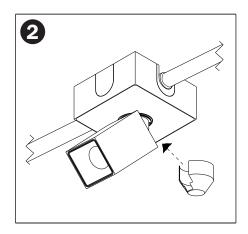
Re-attach and ensure mounting/hinge assembly cover is fully seated and secured in place.
