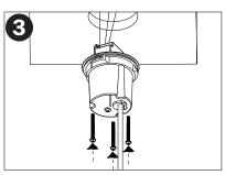
Fasten recessed canopy to junction box mounting plate with supplied fasteners. White line on bottom of recessed canopy indicates direction of square cylinder walls.
