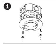
Fasten mounting plate to junction box (by others). **Must be installed prior to ceiling installation.**
