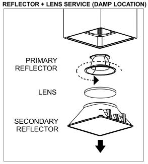
To service or change the reflector lens, rotate the secondary reflector 45° counter clockwise to release. Then rotate the primary reflector 45° counter clock wise to release.
