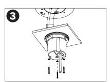
Fasten mounting assembly to the mounting plate with supplied fasteners.
