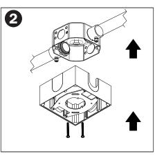
Assemble conduit canopy to junction box through oblong slots with machine screws.
