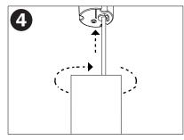
Ensure secondary leads are connected (+)(-) with lever locks. Twist cylinder clockwise to lock to the mounting assembly. If cylinder is not aligned, unlock from mounting assembly, rotate cylinder 120deg and lock again.
