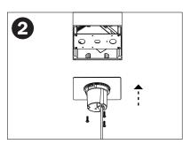
Fasten mounting plate assembly to canopy. If wet location press fit required.
