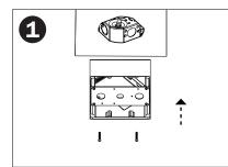
Make primary wire connections. Assemble canopy to junction box through oblong slots with machine screws.
