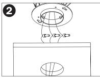
Connect driver leads to supply voltage. Ensure the correct voltage is selected. Refer to "Wiring Instructions" document.
