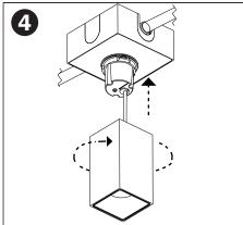
Ensure secondary leads are connected (+)(-) with lever locks. Twist cylinder clockwise to lock to the mounting assembly. If cylinder is not aligned with canopy, unlock from mounting assembly, rotate cylinder 120deg and lock again.
