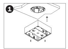
Make primary wire connections. Assemble canopy to junction box through oblong slots with machine screws.
