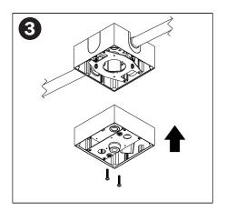
Make supplied connections. Check with wiring diagrams. Place canopy onto conduit canopy and fasten screws through key holes on the canopy's top plate into conduit canopy plate.
