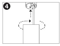
Ensure secondary leads are connected (+)(-) with lever locks. Twist cylinder clockwise to lock to the mounting assembly. If cylinder is not aligned with canopy, unlock from mounting assembly, rotate cylinder 120deg and lock again.
