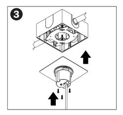
Make supply connections. Fasten Mounting plate assembly to conduit plate inside of conduit canopy with supplied screws.
