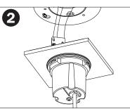
Connect driver leads to supply voltage. Ensure the correct voltage is selected. Refer to "Wiring Instructions" document.
