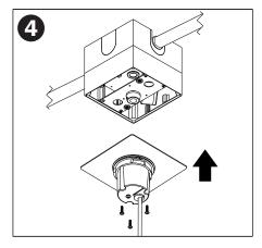
Fasten Mounting plate assembly to canopy bottom plate with supplied screws.
