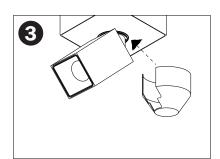
Re-attach and ensure mounting/hinge assembly cover is fully seated and secured in place.
