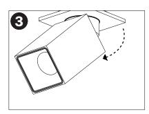
Tilt cylinder to expose mounting/ hinge assembly cover. See C3SAS-3C (Steps 2-4) for remaining steps.
