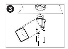
Fasten mounting / hinge assembly to the integral driver junction box mounting plate with supplied fasteners.
