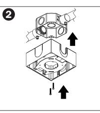
Assemble conduit canopy to junction box through oblong slots with provided machine screws (8-32 x 1.5").
