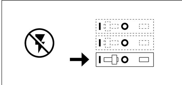
**TURN OFF POWER** before connecting trim. Failure to do so will cause **LED FAILURE**.
