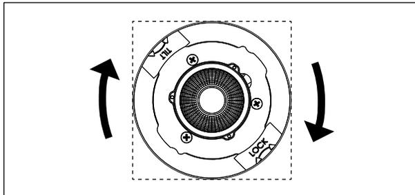
Install the light engine into the internal housing bracket. Twist the light engine 1/4 clockwise to lock into place.
