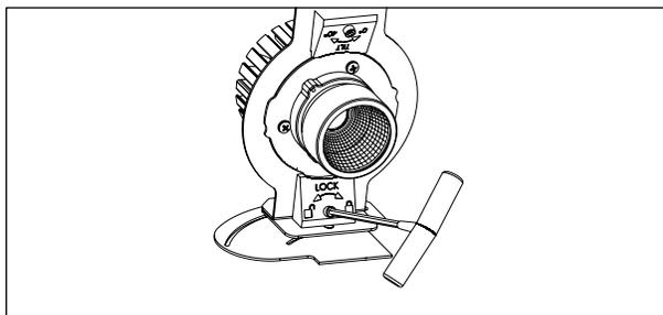
Unlock the tilting mechanism with a 1/4 counter clockwise turn using the 9/64" hex key. Once adjustment is completed (step #4b) lock the tilt mechanism with a 1/4 clockwise turn.
