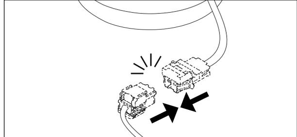
Connect the mating connectors on the light engine and housing.
