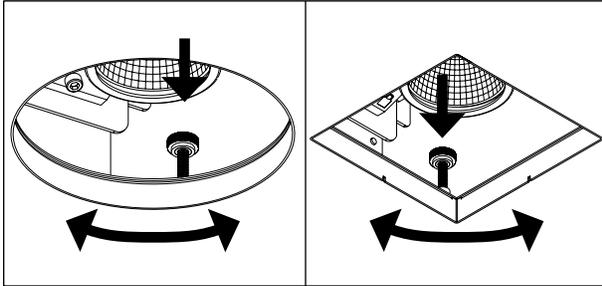
Unlock rotation screw with a counter clockwise turn. Rotate the light engine (361° rotation) to the desired angle. Lock the rotation screw with a clockwise turn.
