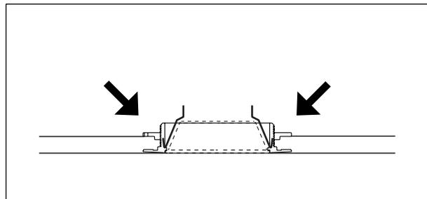
Once passed the ceiling plane, trim clips will expand to lock the trim into place.
