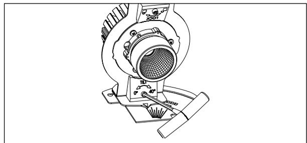
Ensure adjustment lock is disengaged (step #4a). Adjust tilt to the desired angle using the 9/64" hex key. Turn clockwise to tilt. Re-engage adjustment lock (step #4a).
